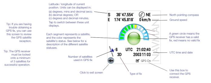
Tip: In practice less than 12 satellites are tracked by the GPS receiver due to satellite positioning. Latitude and longitude are displayed along with a North-pointing compass, the heading in degrees and ground speed.
